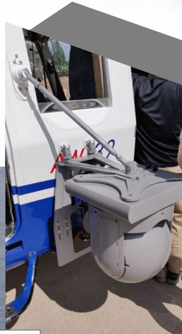
Position of the Camera Support Attachment points
